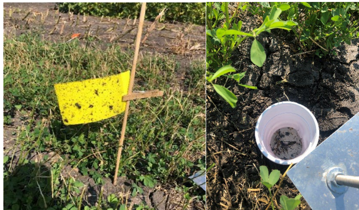
Figure 4.1. Example of sticky trap (left) and pitfall trap with swivel cover off to the side for easy access (right).
