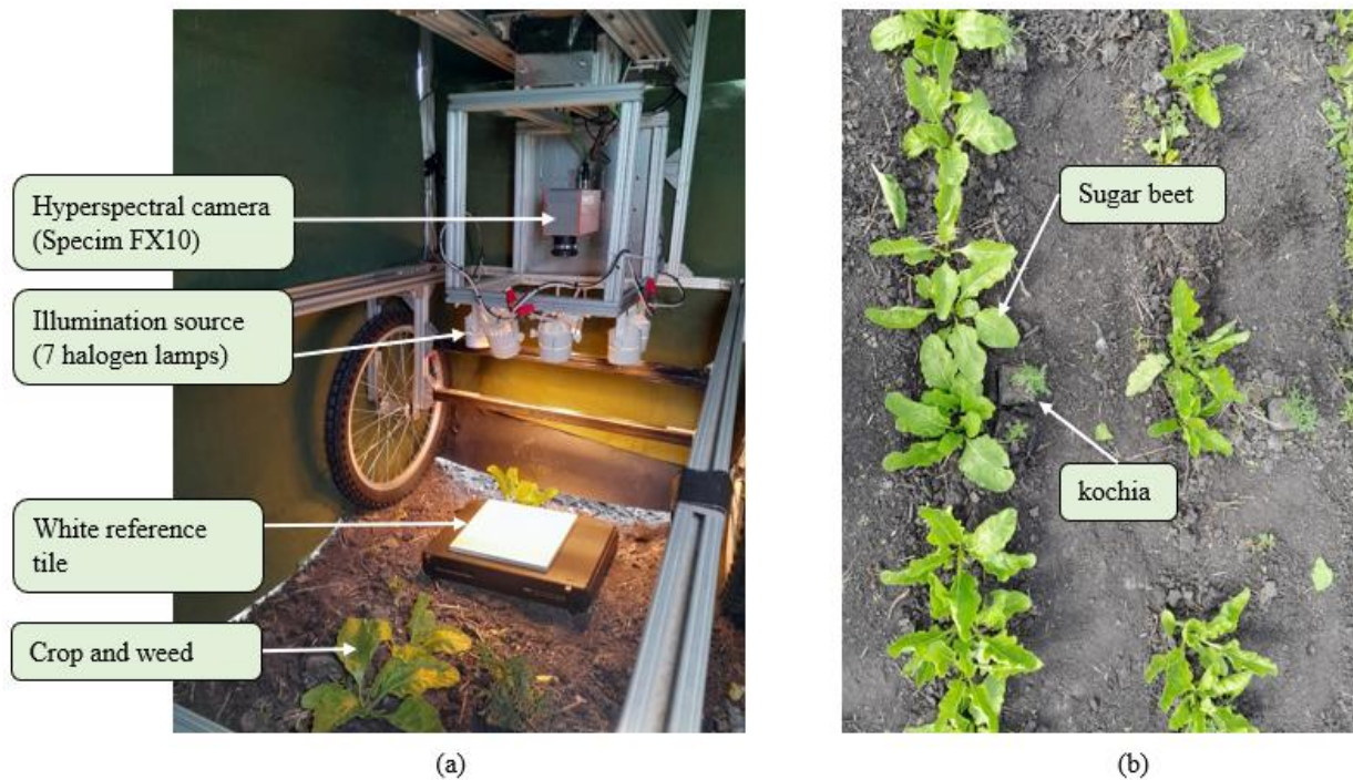
Figure 7. Field data collection (a) hyperspectral sensor mounted on a scanning platform for data collection of raw, white reference and dark reference image (b) raw RGB image.
