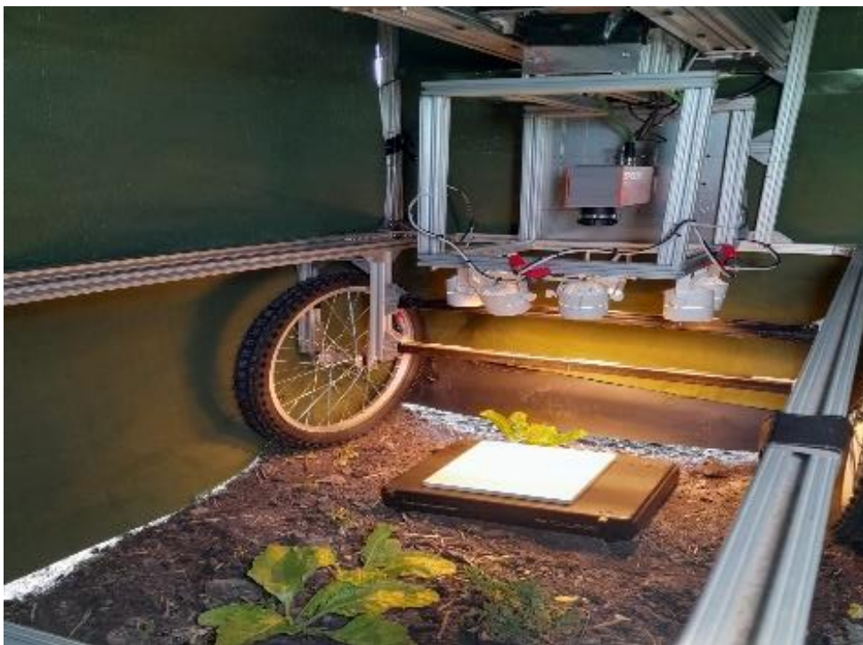
Figure B6. Capturing white reference image and raw image with the sensor with tarp covering the platform to minimize external effects like wind and sunlight.
