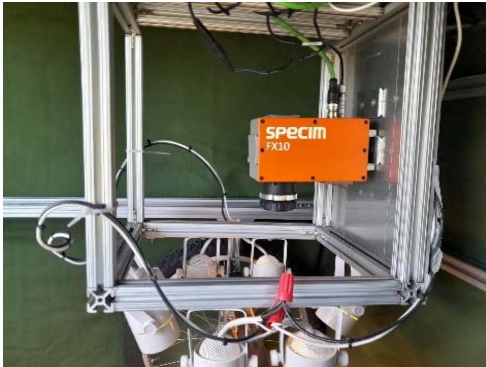
Figure B5. Hyperspectral sensor (Specim FX10) mounted on data collection platform utilized to record images in greenhouse and field.
