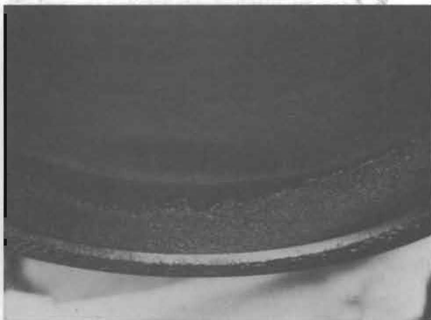
Figure 6. Heavy carbon deposits were found on the liner surface above the top ring land.
