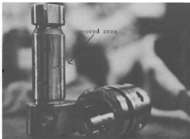
Fig. 4. Failed Injection Pump Parts
