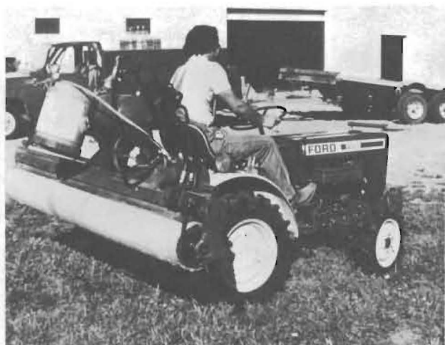
Figure 3. A roller applicator showing the carpet covered roller and the herbicide reservoir.
