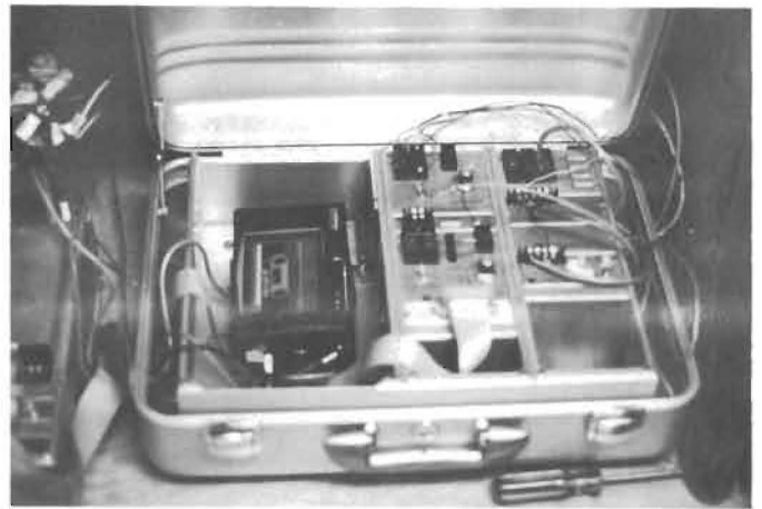
Part of the monitoring equipment used in the energy-integrated farm project. When hooked to another unit measuring various temperatures in the dairy facility, the equipment shown measures wind velocity and direction and water use, and records all the data on a magnetic tape for later use with a computer.
