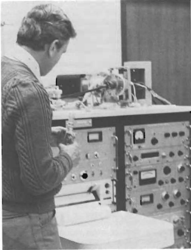
Dr. John Moraghan measures isotope concentrations in nitrogen fertilizers with the mass spectrometer.
