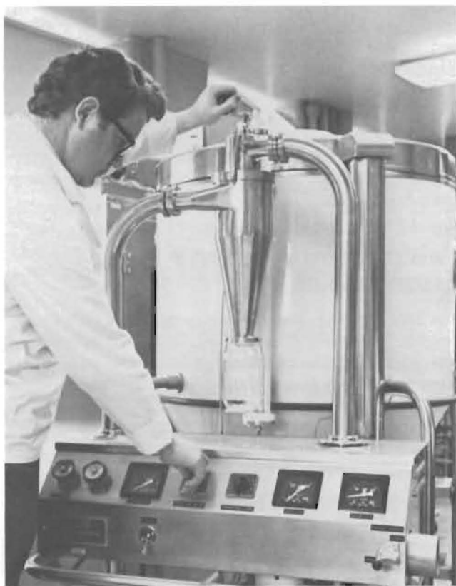
Dr. Brendan Donnelly operates an experimental spray drier for protein preparation from sunflower seeds.
