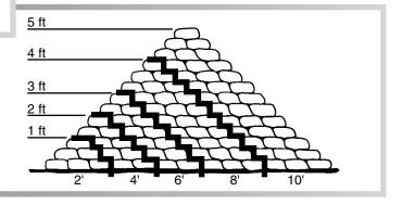
Estimated cubic yards of sand needed per 100 feet of dike length for various dike heights and ratios of height to width. An additional 2 cubic yards will be needed for bags to hold the plastic.
