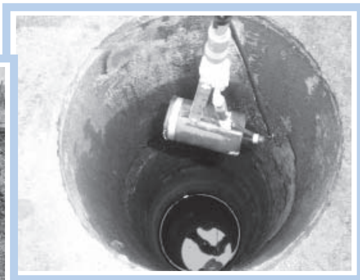
Figure 4. Underwater camera about to be lowered into a well to look for problems in the casing and screen.
