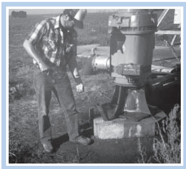
Figure 3. Measuring the water level in a well with a steel tape.
