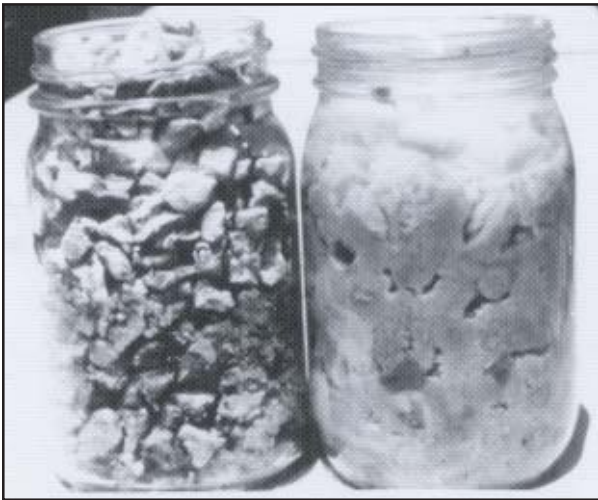
Commercial chipped sodium bentonite (left jar) is a natural clay that expands in water (right jar). Ten feet of bentonite placed near the water table provides additional protection in locations where secondary contamination is a concern.
