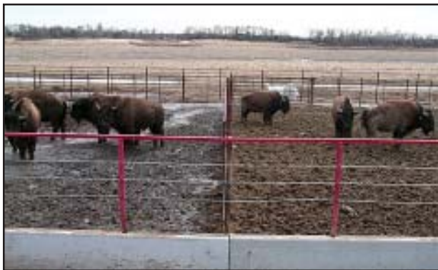
The ash-modified soil in the right pen provides improved drainage and stability, while wet, muddy conditions are evident in the untreated area (left).
