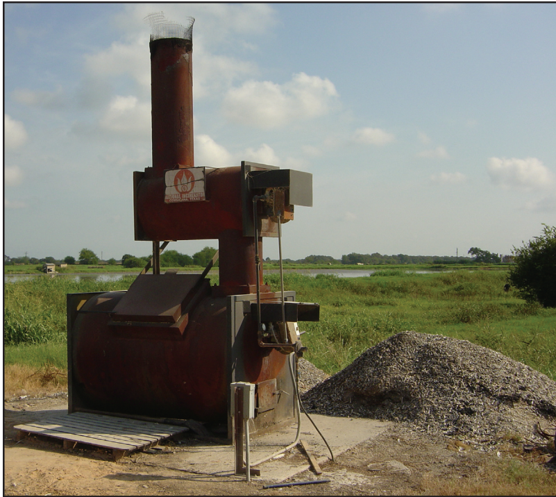
Fig. 1. Incinerator for managing poultry carcasses.
