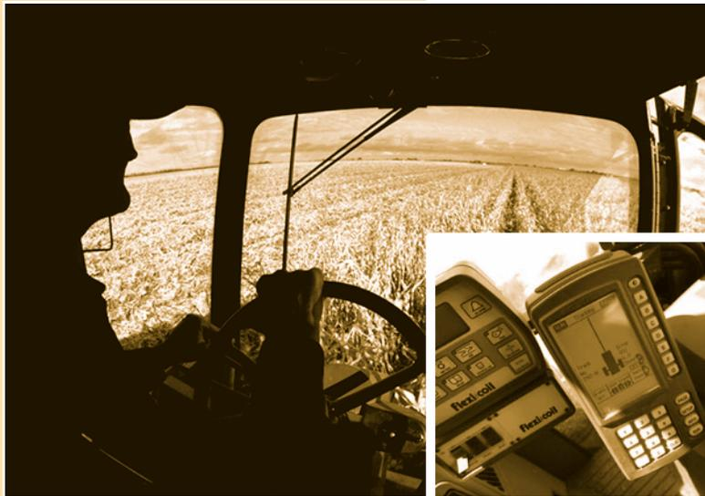
**Figure 1. GPS guidance system in a tractor.**
