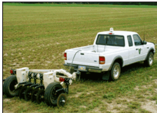
Figure 6. Electrical conductivity sensor and readings from a field east of Crookston.
