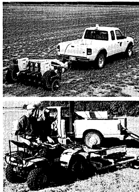
Figure 6. Veris conductivity sensor (top), EM-38 in use. (Norm Procnow and Hal Weiser, USDA-NRCS, Jamestown, N.D.)
