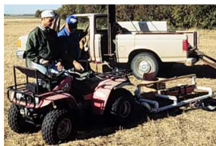
Figure 6. Veris conductivity sensor (top), EM-38 in use. (Norm Procnow and Hal Weiser, USDA-NRCS, Jamestown, N.D.)
