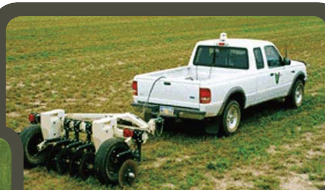
Veris soil EC sensor. (Photo courtesy of Veris Technologies, Salina, Kan.)
