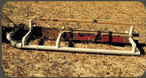
EM-38 being used on a PVC sled near Valley City, N.D.
