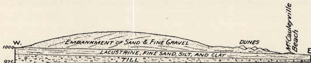
FIG. 19.—Section across the Campbell embankment in sections 20 and 21, township 161, range 55. Horizontal scale, one-third of a mile to an inch; vertical scale, 100 feet to an inch.
