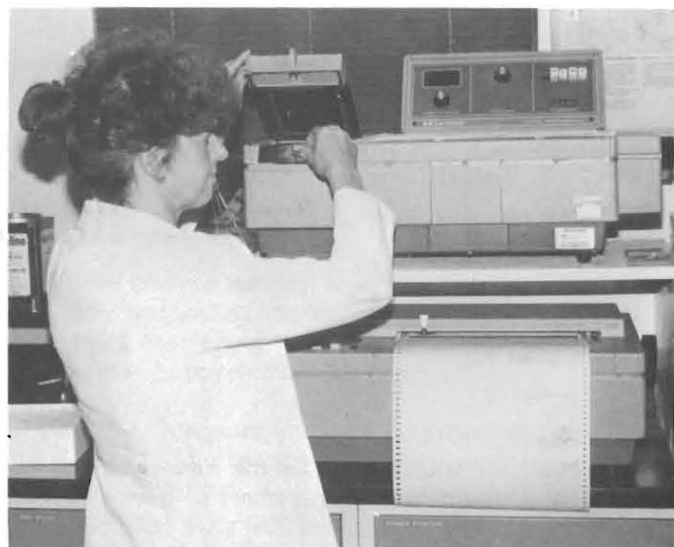
Microbiology technician Carolyn Maier measures enzyme kinetics on a spectrophotometer, studying microbial metabolism and how microbes change food.
