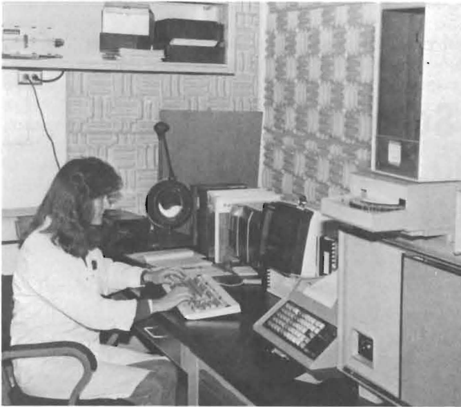
Beth Kornelius works at a mass spectrometer in the toxicology laboratory. Used to identify organic materials, the spectrometer produces "fingerprints" of pesticides and other compounds.
