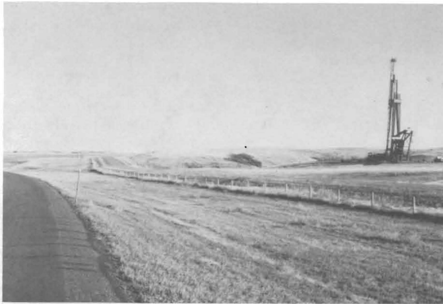
This oil and gas well, just south of I-94, has been directionally drilled into subsurface park lands north of the interstate.
