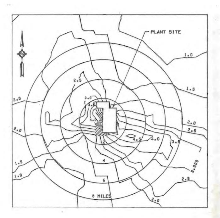
FIGURE 3-2 ISOPLETHS OF ANNUAL AVERAGE NO<sub>X</sub> CONCENTRATION (µGM/M<sup>3</sup>) FROM METEOROLOGICAL DATA FOR BISMARCK, NORTH DAKOTA ISOPLETH INTERVAL 0.5µGM/M<sup>3</sup>
