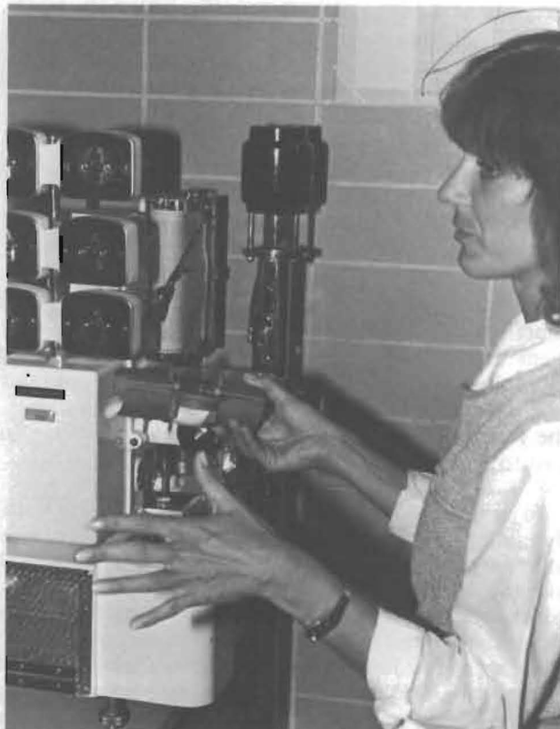
A cereal chemistry department lab technician demonstrates how an extensograph measures gluten strength by measuring a dough's extensibility and resistance to extension.
