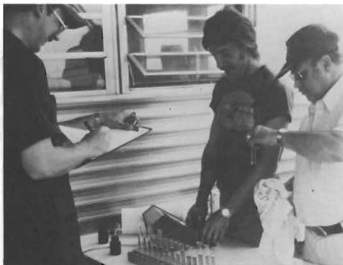
Figure 2. The change of color of the copper tracer is analyzed with a colorimeter to give a digital readout.
