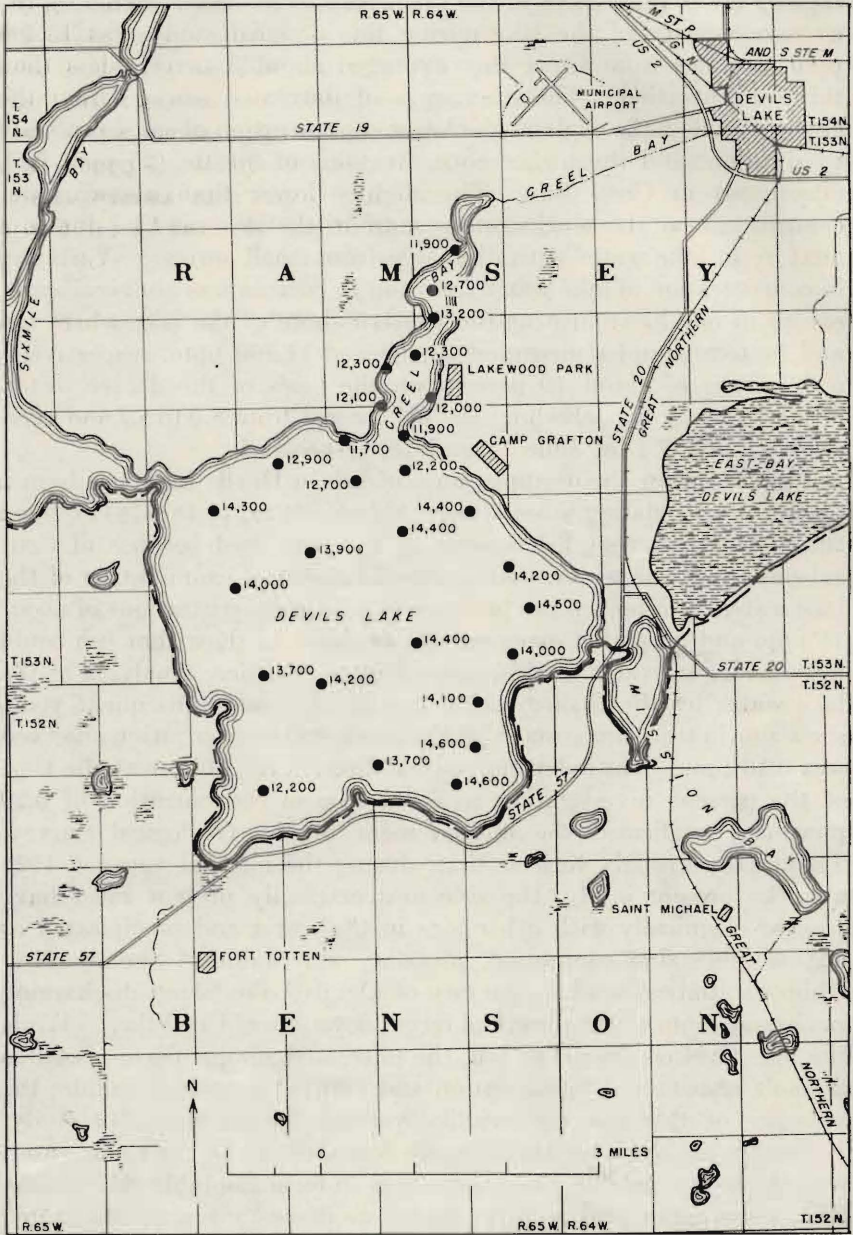
Figure 12.—Map of Devils Lake showing areal concentration of salts in parts per million, June 14-18, 1949
