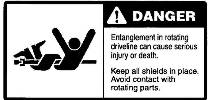
Figure 2. Danger. Indicates one of the most serious potential hazards. Usually red with black or white text on white or black background.
