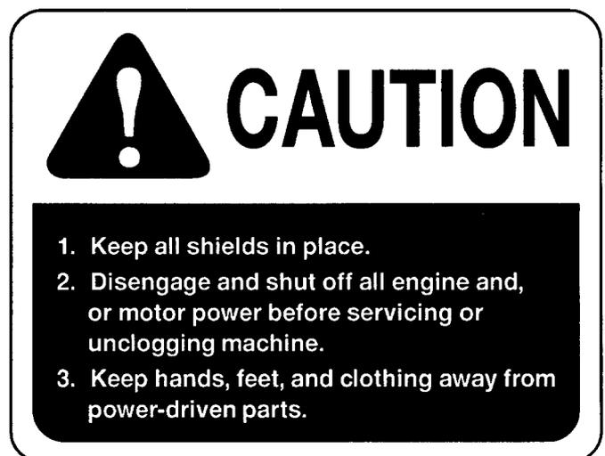
Figure 4. Caution. Intended to remind workers of safety instruction and identify a hazard less serious than those indicated by Warning. Usually yellow with black or white text on white or black background.
