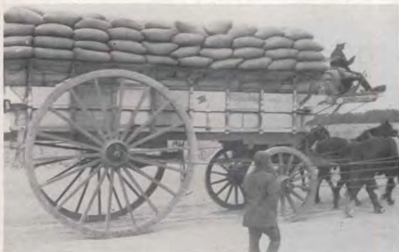
Typical 16-horse "carro", capable of hauling more grain than the best truck and its trailer. This one was seen near Tres Arroyos.
