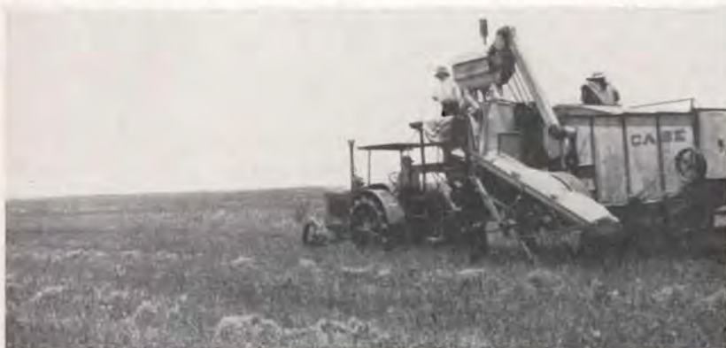
Modern Deering tractor and Case combine dropping off a consignment of bags. Two men stand on platforms; one does the sewing.
