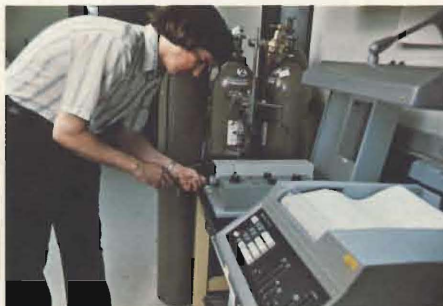
Dr. Paul Holmes uses gas chromatography to help identify the various kinds of psychrophilic anaerobic bacteria that break down waste materials in solid waste disposal systems.
