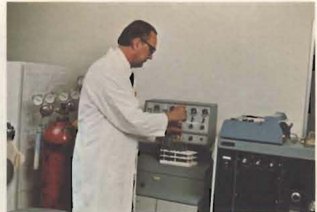
Dr. Berdell R. Funke tests the effects of pesticides on nitrogen fixation by legumes. He uses a gas chromatograph and a technique known as acetylene reduction.
