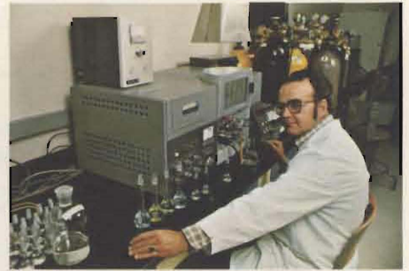
Dr. Howard Casper is able to measure the amount of lead or mercury in animal tissues through this atomic absorption spectrophotometer. Such analysis helps determine some specific poisons that cause death in farm animals.
