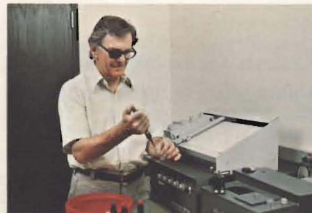
Dr. Bayard Sleeper works with a recording spectrophotometer to identify the enzymes involved in bacterial nitrogen metabolism, searching for the reasons why flaxseed meal is toxic to farm animals.
