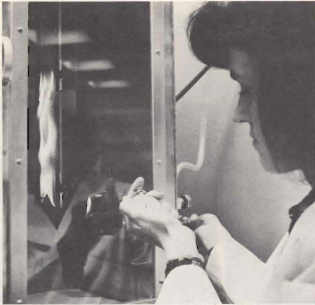
Flame is removed from sample after three seconds. Mrs. Meyer observes residual flame time and char length for each specimen.
