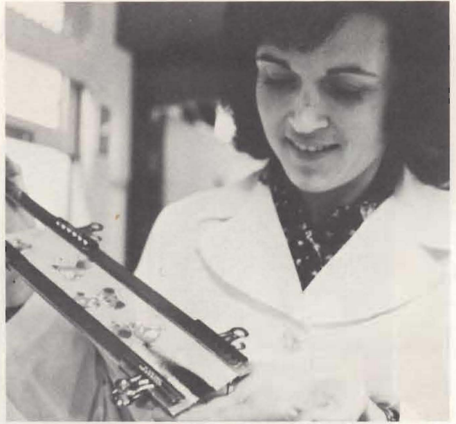
Cotton flannelette fabric with flame retardant finish has self-extinguished after three seconds of exposure to flame.
