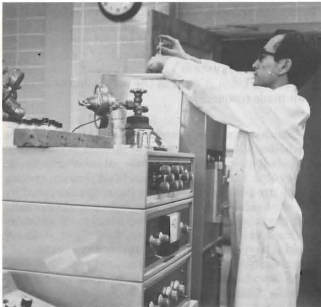
Graduate student Sung-kon Kim determines the fatty acid composition of wheat fat on the gas chromatograph.
