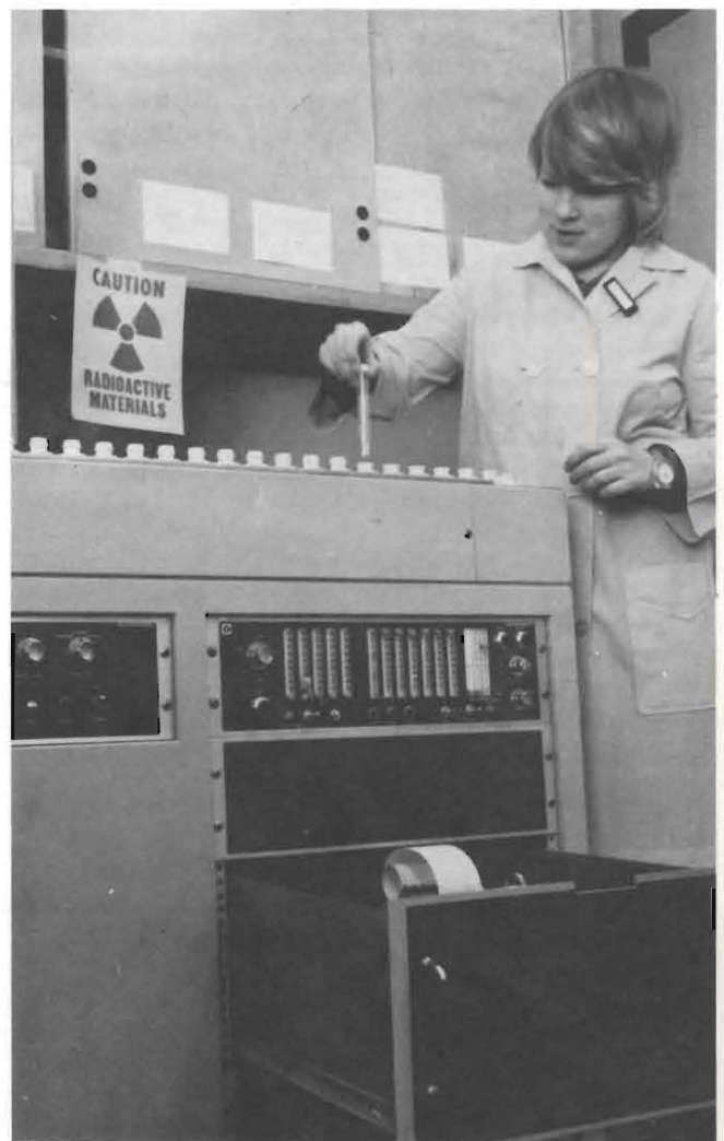
Sandy Matz, animal science technician, traces animal metabolic processes by means of this gamma radiation counter.
