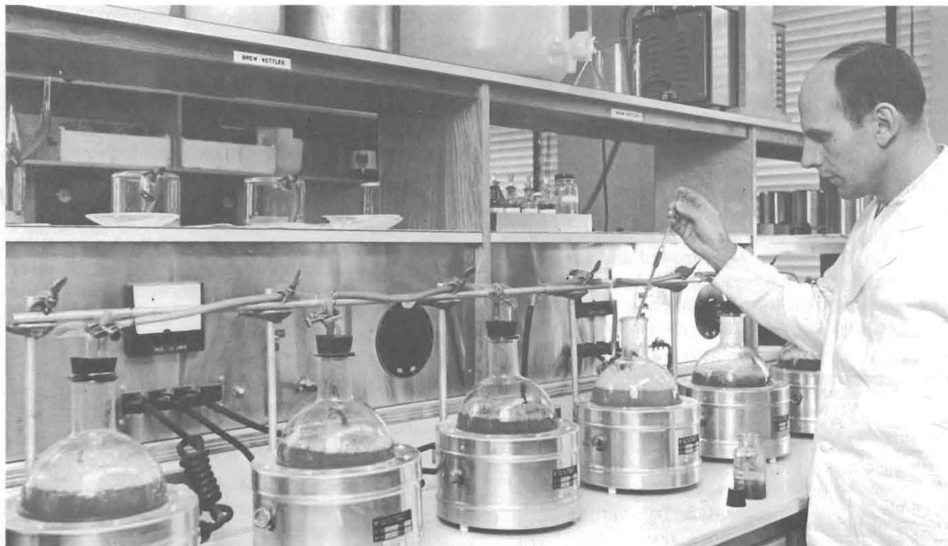
Fig. 3. During the bottle boil, Evan Cummings adds hop extract which is the main flavor component of beer.
