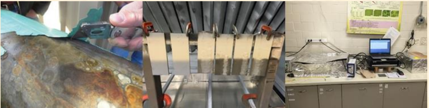
Self-sensing thermally sprayed metallic coatings for pipeline corrosion mitigation and assessment (L to R): an example of pipeline corrosion, thermally sprayed metallic coating samples with sensors embedded, and laboratory corrosion test setup.
