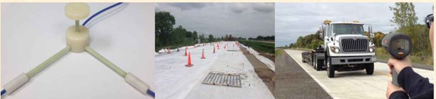
Innovative fiber optic sensors for pavement monitoring (L to R): a sensor, installation, and field testing at MnROAD, MN.
