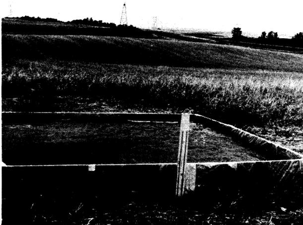
**Figure 1. Flooded basin on a plot to measure water movement into and through the reconstructed "soil".**
