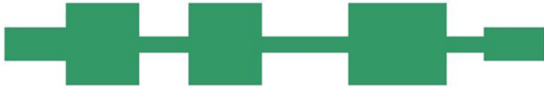
(c) Microstrip-line filter layout.
