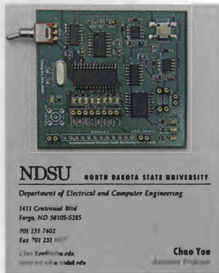
Figure 5. Actual size of the sensor node
