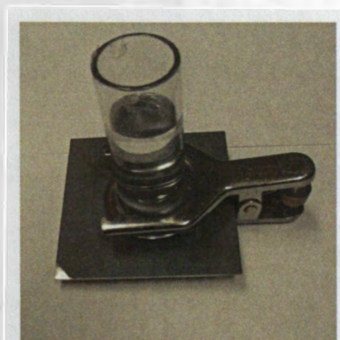
Figure 18. Mg-rich primer with ANAC topcoat coating sample
