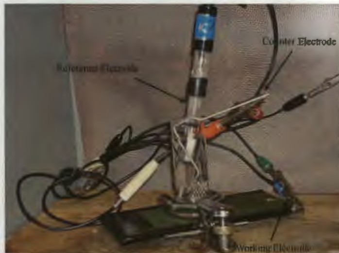
Figure 20. Real picture of the EIS electrodes connection
