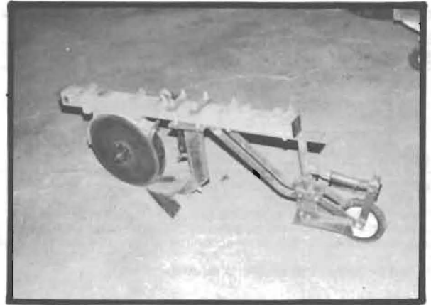
Figure 4. Modification number 3, showing the double disk furrow operators mounted in front of a 12" sweep followed by the seeding assembly with fins and pack wheel attached.
